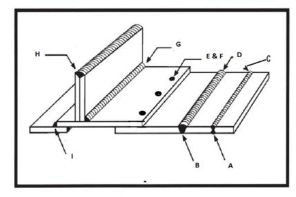
A) Oxy-Fuel cut in half then prepare bevel B) Oxy-Fuel double bevel C) 7018 Weld 1G 3/32 Weld Crown 1/8 Gap D) 7018 Weld 3G 3/32 Weld Crown 1/8 Gap
